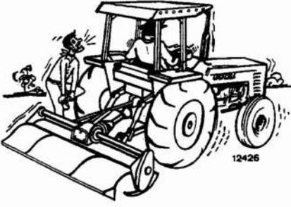
■ Never operate a PTO driven implement without first ensuring that no one is on or near the machine. Check that all rotating parts connected to the PTO shaft are adequately protected.
