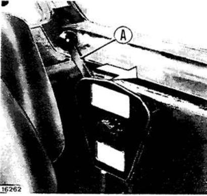
This special hook permits towing of implements, agricultural machines and trailers provided with eye couplings. Additionally, any hitching/unhitching operation can be done from the Operator's seat.
